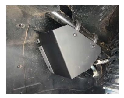
Once in place slide the guard back down the frame into location so that the small plastic
