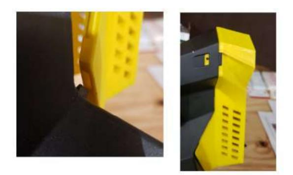
• Install the supplied screw and washers as seen in the picture below. Do not overtighten these as it will cause the part to break in most cases. It takes very little tightening to get the covers to be sturdy for this design.
