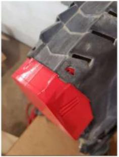
• Install the supplied screws and washers as seen in the picture below. Do not overtighten these as it will cause the part to break in most cases.
