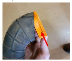
• While pushing up on the insert push the bottom of the insert into the bottom of the snorkel intake. Only press along the outsides of the insert, pressing on the screen/mesh may cause the mesh to break.
