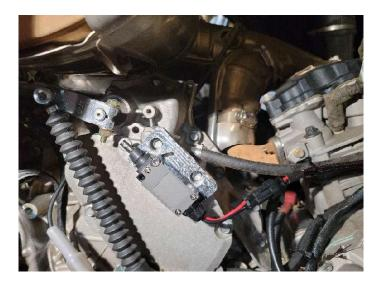
• If the bolt seems like it is to long and binding on the switch while shifting into reverse add the supplied washers to the bolt head side of the shifter linkage bolt.
