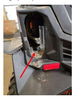
• Re-install the tail light using the original bolts taken out and then plug the OEM tail light plug into the tail light and connect the yellow wire from the supplied reverse light harness to the yellow plug on the tail light. Push the rear plastic back into place and re-install the screws at the top of the bed.
