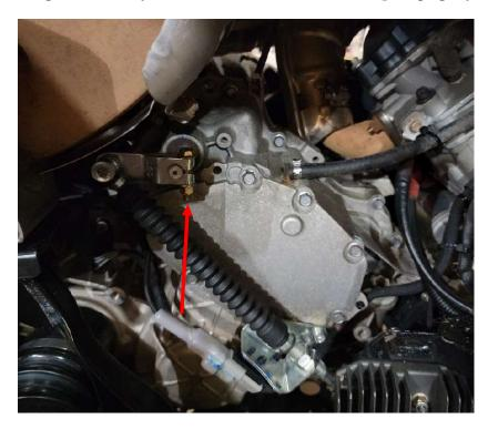
• Slide the switch to the bottom of the bracket to have the best access to the mounting bolt holes.
