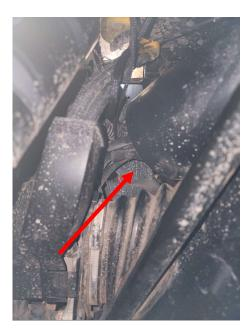
• Feed the open plug ends of the cage harness up through the bottom of the driver side front cage pillar. Use the slots in the side of the pillar to help run the wire up to the top exit hole.
