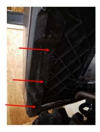
• Remove the side screws from the box side panel Both passenger and driver side.
