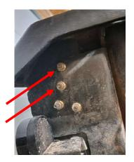
• Install the new latches using the removed hardware and re-install the side panels in the opposite order of the removal steps.
