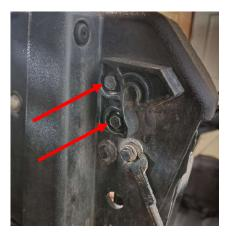
• Using a 10mm wrench and 10mm socket remove the two mounting bolts and nuts.
