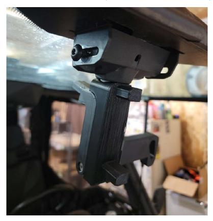
• Close the window and put the handle in the latched position. Push down with moderate pressure and tighten the mount bolts. Open and close the window to insure proper operation.
