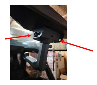
• Turn the handle so the roll pin is lined up with the hole in the bottom of the handle mount. Remove the roll pin from the handle, and remove the washer. (We found the best tool to pinch and remove roll pin is a side snips)
