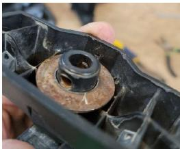
• Install the roll pin the same way as removal by lining up the holes. Check to be sure that the handle still spins somewhat freely. If it is to tight initially do not force it as this may cause the handle end to break. If this is the case you will need to remove one of the shims.
