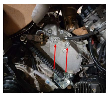
• Remove the top two bolts from the transmission shown in the picture below.
