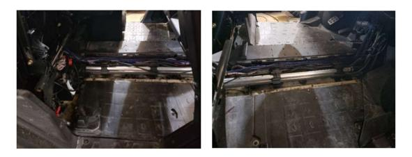
• Run the switch wire down along the gas tank following the OEM wires and through the firewall and then up the center of the machine.
