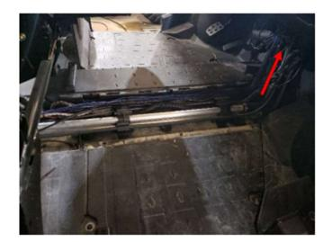
• For Limited Models Find the OEM bullet electrical Connectors in center floor by the heater and attach the wires of the reverse light harness to two of the plugs. Note what color wire and color strip each wire is attached.
