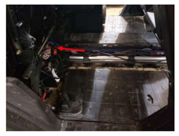
• For non limited models Run the main wire up through the bottom of the dash and up to the rocker switch. Connect the wires per the switch instructions.
