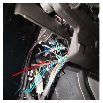
• Attach your accessory to the supplied plug end and test the product. Once operation is verified tie up all loose wires using the supplied zip ties.
