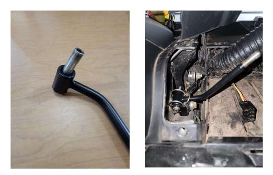
• Reinstall the plastic shift gate and make sure the shifter functions as it should. Install the lock nut and shift handle.
