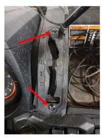
• Loosen and remove the bolt that holds the stock shifter. When removing take note on the orientation of the spring and how it locks onto the bracket to keep tension on the shifter. It will need to be installed in the same way so functionality remains the same.
