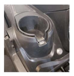
Wedge the screw driver in the rear part of the stock insert and pry up to release the mounting tabs. In most cases the mounting tabs will break off.
