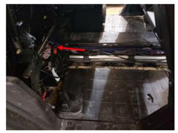
• Run the switch wire down along the gas tank following the OEM wires and through the firewall and then up the center of the machine.
