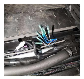
• Remove the dash switch panel by gently pulling the bottom side toward you. Then the top should unhook to give you access to behind the panel wiring.
