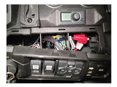
• Attach the bullet electrical connectors to the OEM harness bullet connectors under the dash. Be sure the attach the red and black wires to the same color wires as below in the floor.
