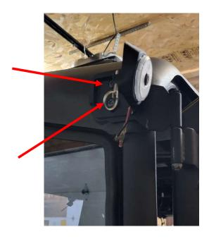
$\circ$   $\,$  Once installed run the wires through the rear window seal or next to cage by the roof.
